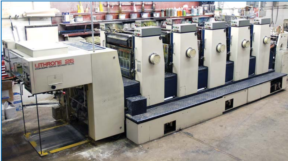
KOMORI LITHRONE 26, MODEL L-526-II, 5 COLOUR 20" X 26" PRINTING PRESS
