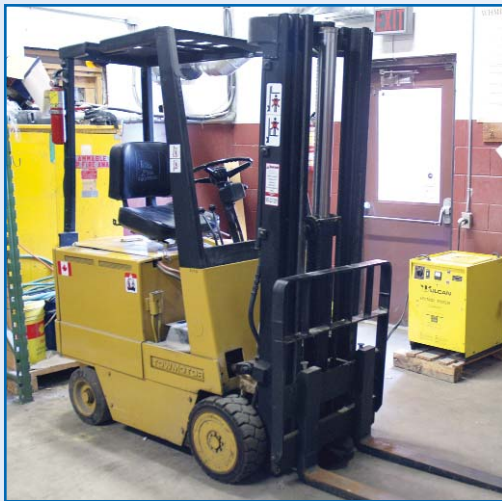
TOWMOTOR ELECTRIC FORKLIFT, 2,100 LB CAPACITY
