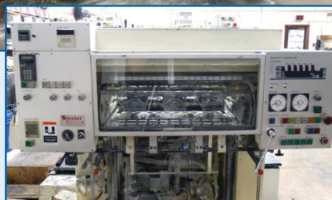
KOMORI LITHRONE 26, MODEL L-526-II, 5 COLOUR 20" X 26" PRINTING PRESS
