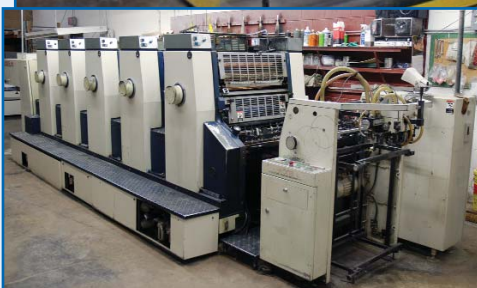
KOMORI LITHRONE 26, MODEL L-526-II, 5 COLOUR 20" X 26" PRINTING PRESS
